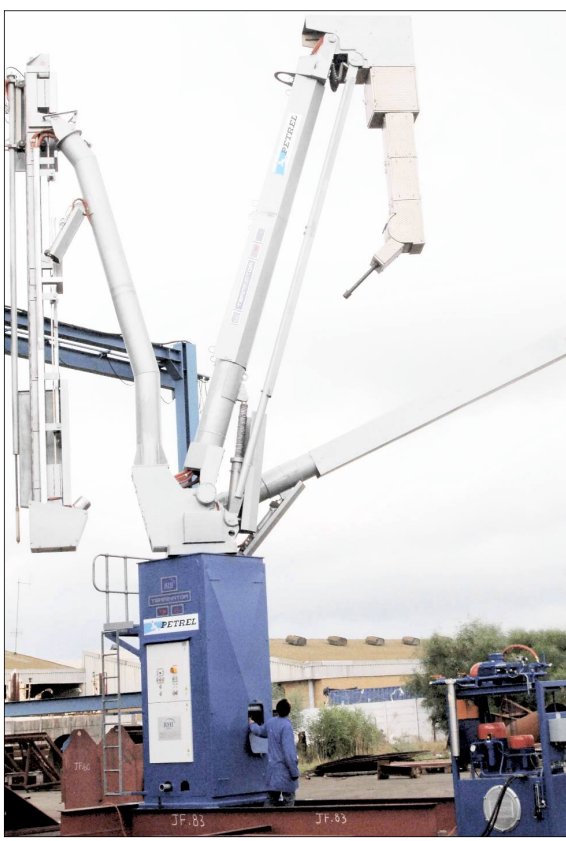
ABOVE: Jorge Cea of ASMAR, Chile and Vincent Chetty, former MD of Petrel, conclude the deal to supply deck equipment. RIGHT: Furnace re-lining machine with laser camera, temperature sensing and gunning booms.
